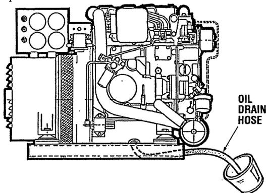
2. **Replacement of the Oil Filter.** When removing the used oil filter, you may find it helpful and cleaner to punch a hole in the upper and lower portion of the old filter to drain the oil from it into a container before removing it. This helps to lessen spillage. A small style automotive filter wrench should be helpful in removing the old oil filter.
