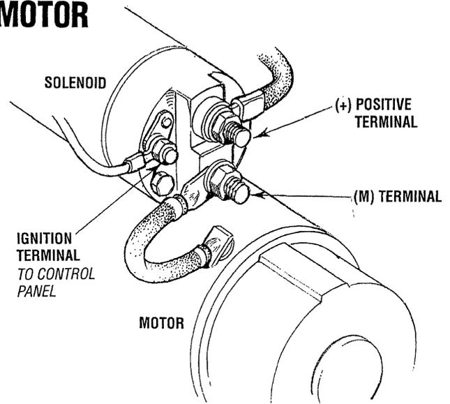
To test the ignition circuit, locate the ignition(s) terminal (it is one of the small terminal studs and is wired to the ignition circuit). Use a screwdriver, don't touch the blade, to jump from that ignition terminal to the positive battery connection terminal on the solenoid.
