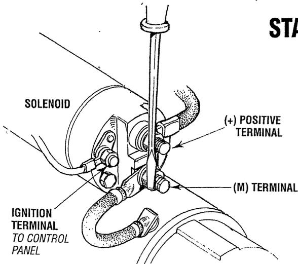
Test again by jumping the two large terminal studs. Hold the screwdriver blade firmly between the studs. Do not allow the screwdriver blade to touch the solenoid or starter casing, this would cause a short.
