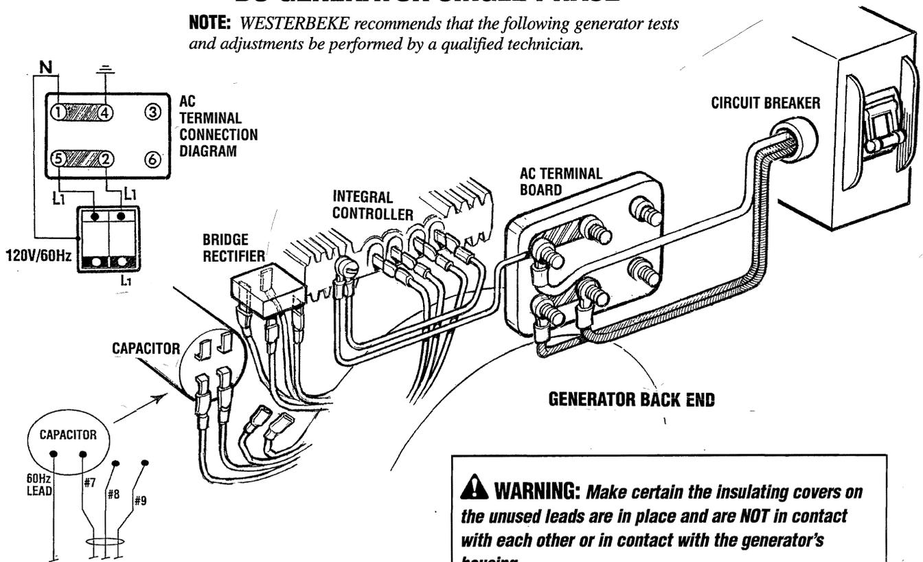
**⚠ WARNING:** Make certain the insulating covers on the unused leads are in place and are NOT in contact with each other or in contact with the generator's housing.
