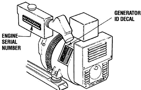
**NOTE:** A carbon monoxide warning decal has been provided by WESTERBEKE. Affix this decal in a visible position in the engine room.
