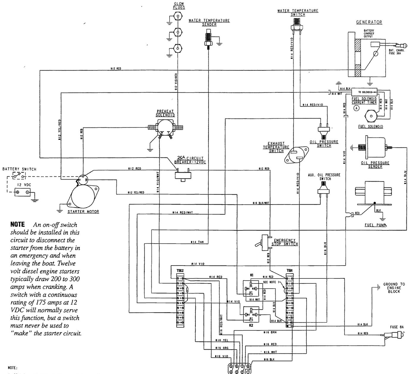
**NOTE** An on-off switch should be installed in this circuit to disconnect the starter from the battery in an emergency and when leaving the boat. Twelve volt diesel engine starters typically draw 200 to 300 amps when cranking. A switch with a continuous rating of 175 amps at 12 VDC will normally serve this function, but a switch must never be used to "make" the starter circuit.
