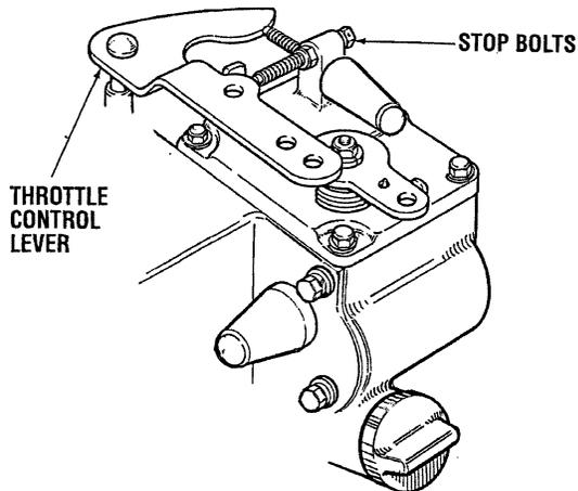
3. To arrive at the appropriate frequency, either monitor the speed of the engine/generator with a tachometer, or monitor the frequency with a frequency meter, the latter method being the more precise of the two.
