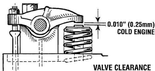
Adjust the valves in #1 cylinder for both intake and exhaust. Proceed to the next cylinder in the firing order.
